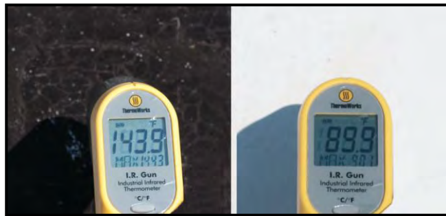
Figure 1: Dark vs. Cool Roof Surface Temperatures
